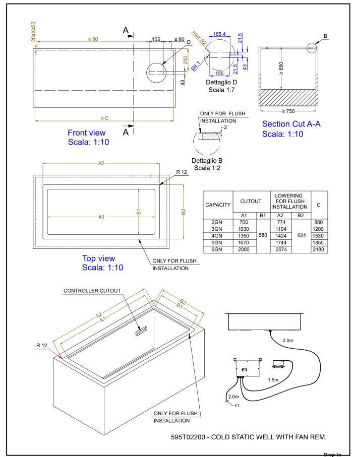
Drop-in remote refrigerated well, static with fan (2 GN container
